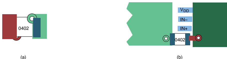
Figure 22. Typical Decoupling Capacitor Layouts
