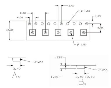
Ao =Change this pocket dimension from 3.4mm to 3.6mm Bo = Change this pocket dimension from 3.4mm to 3.6mm
