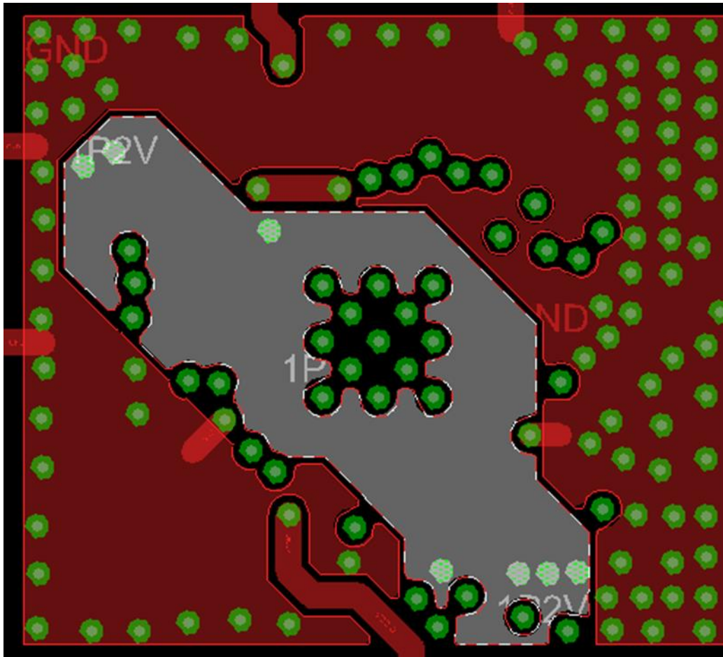
Figure 3-7. Routing of 1P2V Supply
