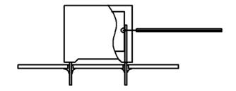
Temperature monitored inside the capacitor.
