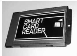
Contact type reader/writer (LR550R03) • High-speed data communication • PC card interface Type II
