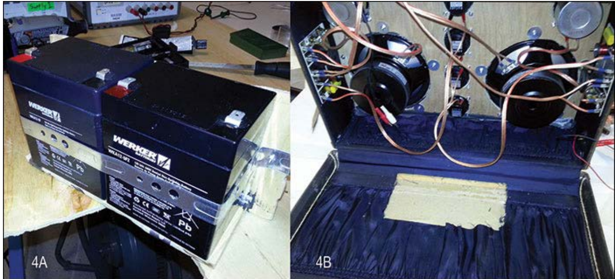
Figure 4. Batteries in the holster (4A). Some of the suitcase lining was removed to accommodate the battery holster, which was placed in the bottom and back of the case to counterbalance the weight of the speakers (4B).
