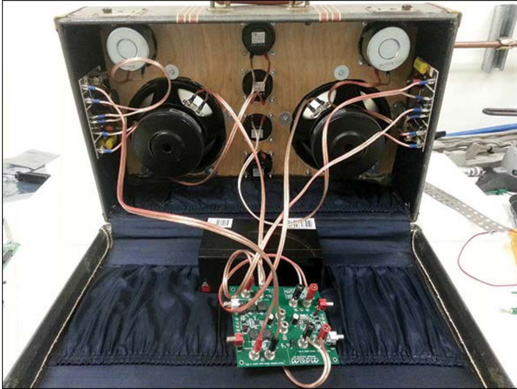
Figure 3. I used 12-gauge speaker wire (overkill, I know) and banana jacks to connect the speakers to the board. I also glued the crossovers to the suitcase walls.
