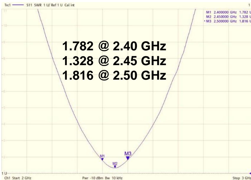
Antenna VSWR on Type-1 Test Board
