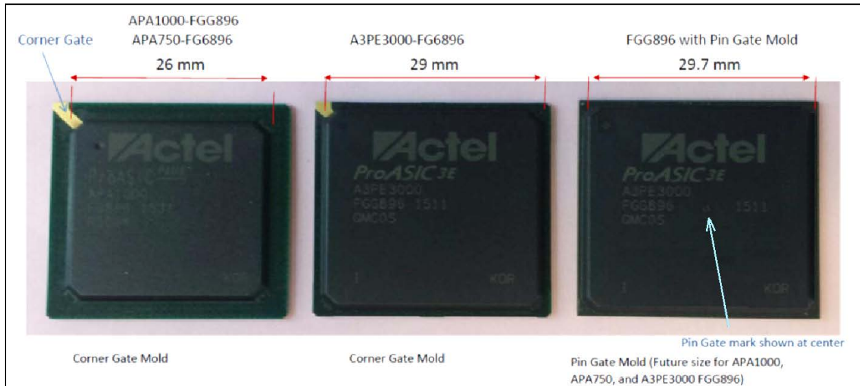
Figure 1 Comparison of FGG896 packaged devices that use the Corner Gate Mold (left and center), and the Pin Gate Mold (right)
