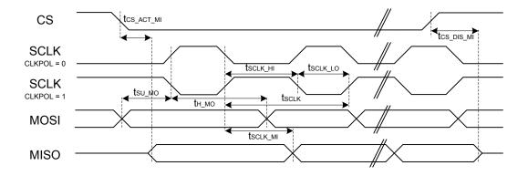
Figure 4.2. SPI Slave Timing Diagram
