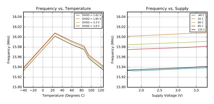
Figure 4.12. HFRCO and AUXHFRCO Typical Performance at 16 MHz
