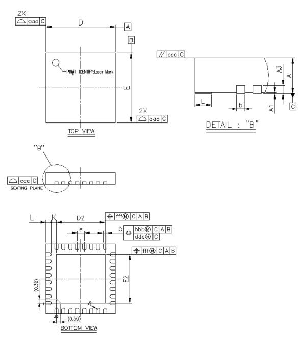
Figure 8.1. QFN32 Package Drawing
