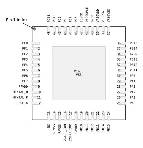
Figure 6.2. QFN48 2.4 GHz Device Pinout
