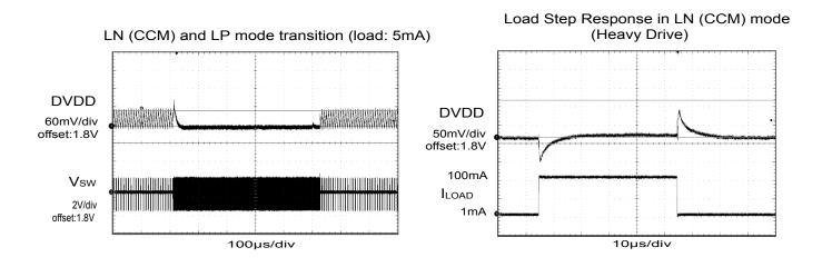
Figure 4.7. DC-DC Converter Transition Waveforms
