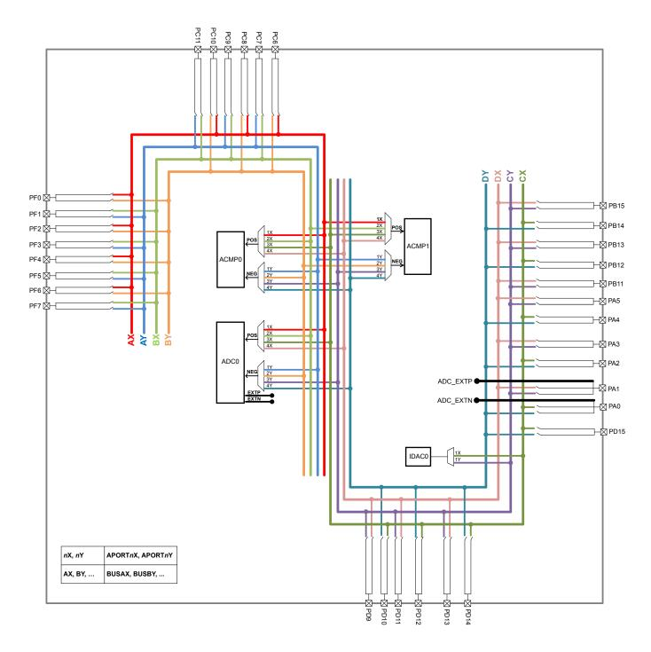
Figure 6.5. APORT Connection Diagram
