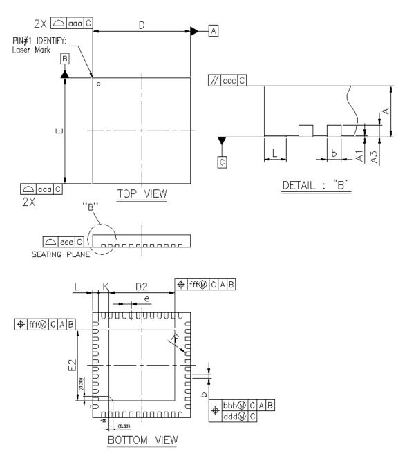
Figure 7.1. QFN48 Package Drawing
