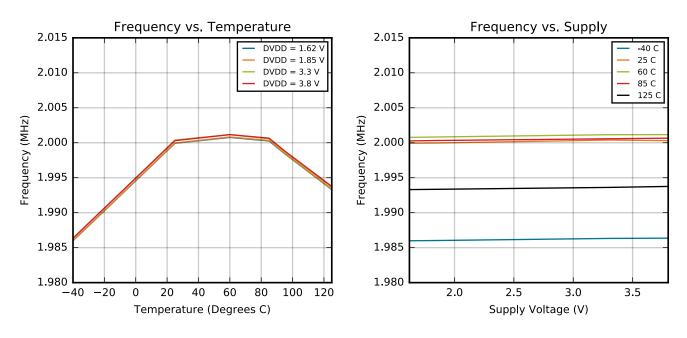
Figure 4.16. HFRCO and AUXHFRCO Typical Performance at 2 MHz
