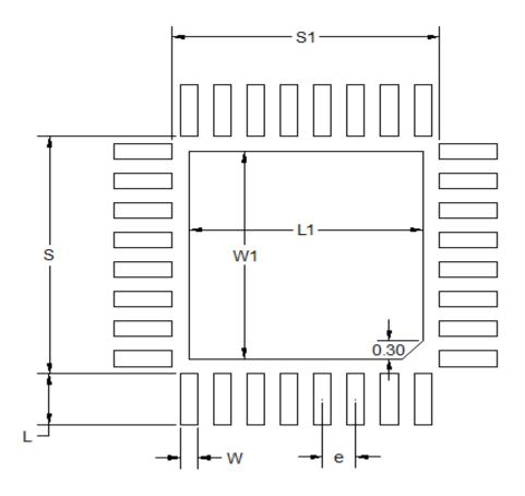
Figure 8.2. QFN32 PCB Land Pattern Drawing
