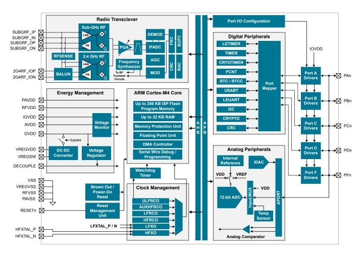
Figure 3.1. Detailed EFR32MG1 Block Diagram
