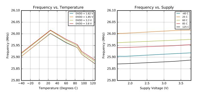
Figure 4.10. HFRCO and AUXHFRCO Typical Performance at 26 MHz
