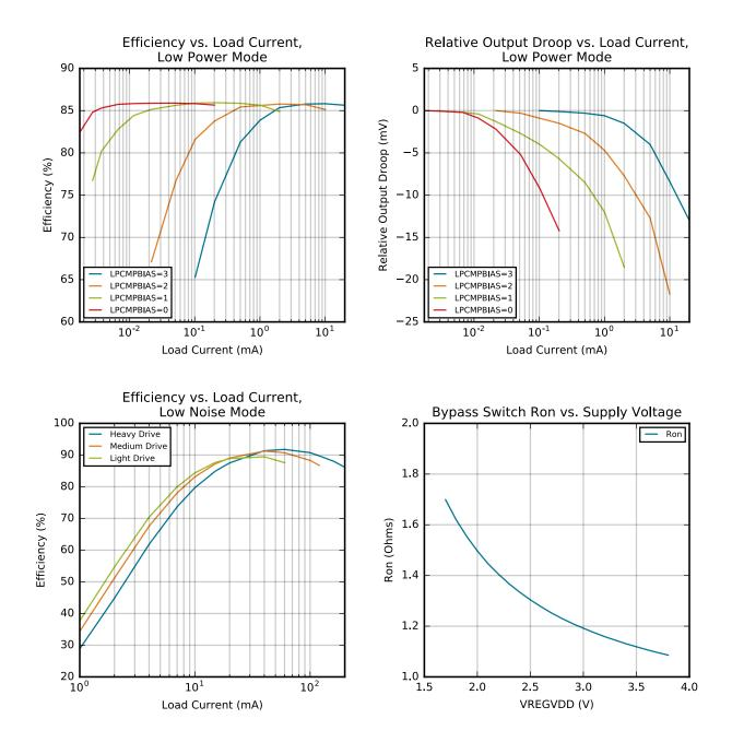
Figure 4.6. DC-DC Converter Typical Performance Characteristics
