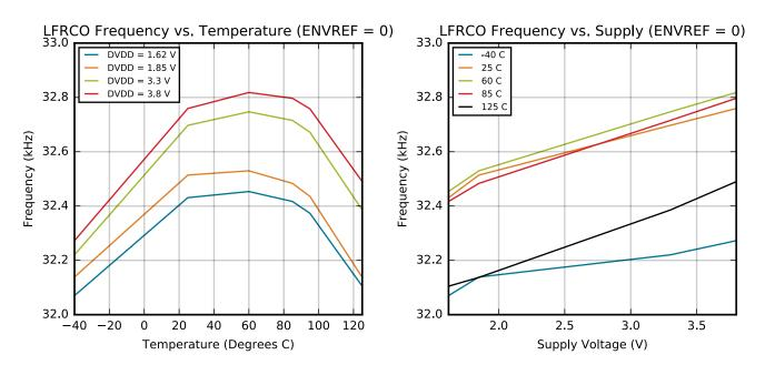
Figure 4.18. LFRCO Typical Performance at 32.768 kHz
