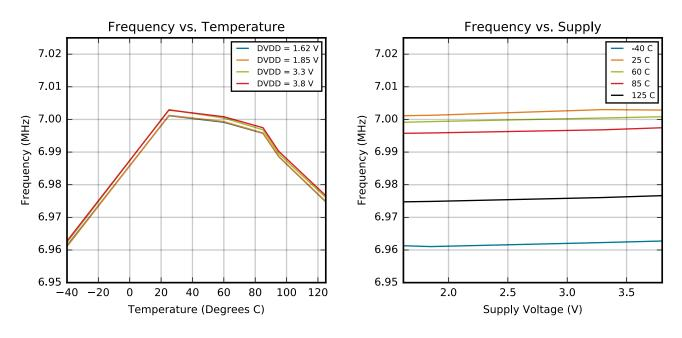
Figure 4.14. HFRCO and AUXHFRCO Typical Performance at 7 MHz
