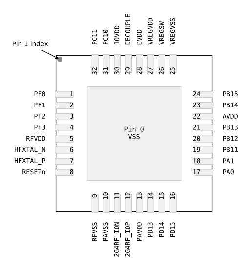
Figure 6.4. QFN32 2.4 GHz Device Pinout
