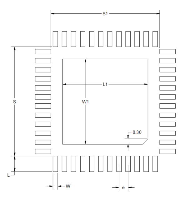
Figure 7.2. QFN48 PCB Land Pattern Drawing
