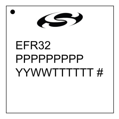
Figure 7.3. QFN48 Package Marking
