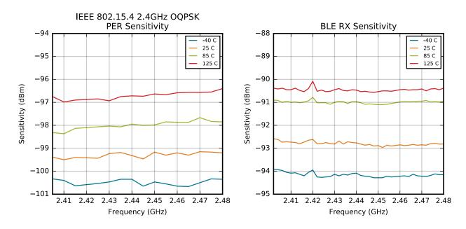
Figure 4.21. 2.4 GHz RF Receiver Sensitivity
