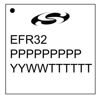
Figure 8.3. QFN32 Package Marking
