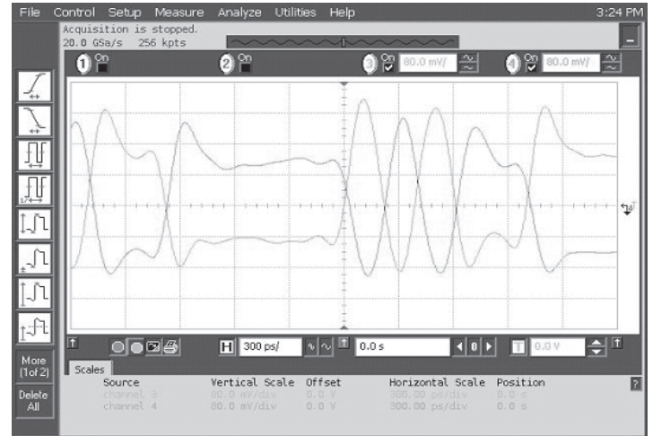
Data Waveforms, 3.0Gbps (left) & 6.0Gbps (right)
