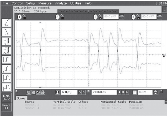
Data Waveforms, 3.0Gbps (left) & 6.0Gbps (right)
