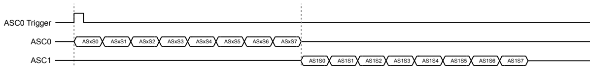
Figure 17-5. ASCx, ADCCTL.ADCMODE = 011b, 110b
