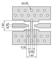
Line width be designed to match  $50\Omega$  characteristic impedance depending on PCB material and thickness.
